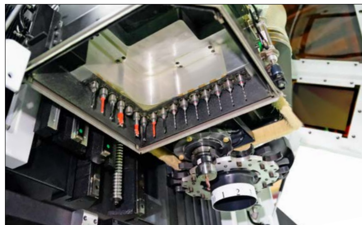
10-tool Carousel with PMM System Various Boring Unit types With L Shape
