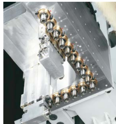
The boring unit is equipped with 16 vertical spindles and two 2-way-spindle unit for horizontal drilling.
