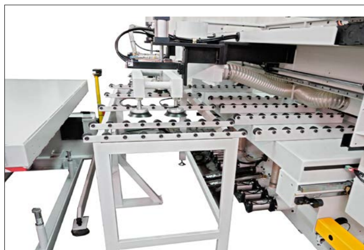
Roller System for loading panels
