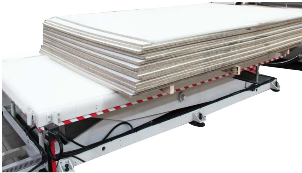
Hydraulic Lifting system Loading for panels up to 2 tons
