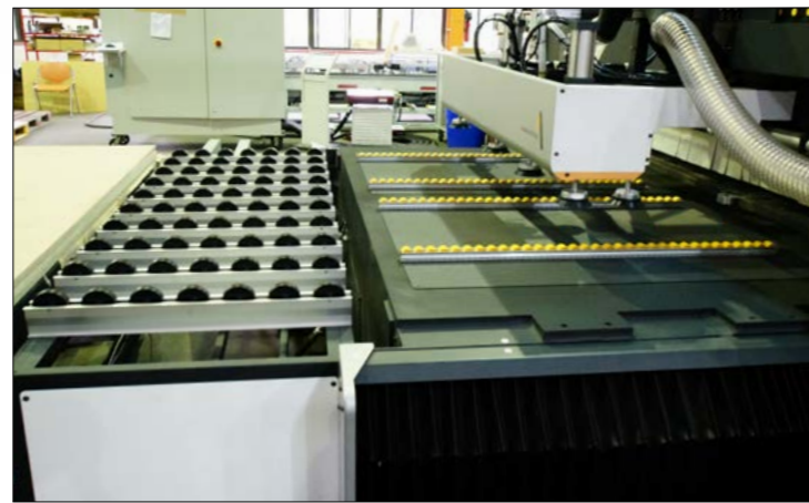
Roller System for loading Panels
