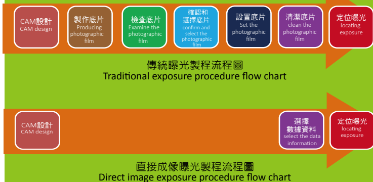
圖二，傳統與直接成像曝光製程流程圖 Fig.2. Traditional and direct image exposure procedure flow chart
