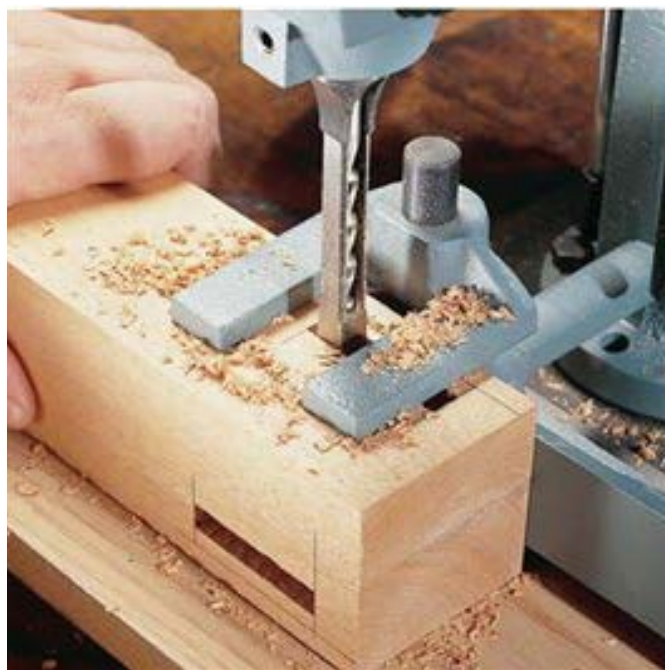
圖四：重疊數個正方形孔形成一個長方形的榫孔 (3) Fig.4 Overlapping several square holes to make a rectangle mortise hole [3]
