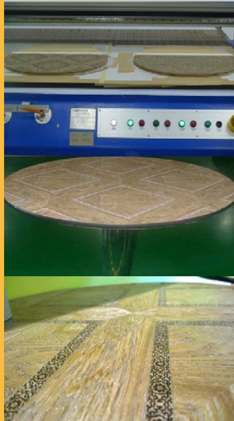
密集板貼 PVC 後，UV 直噴 3D 堆疊 Medium Density Fiberboard after pasting PVC, UV direct spray 3D stack
