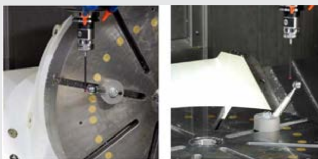
Fig 8 SIEMENS使用cycle996功能配合量測儀器進行旋轉機構設定 Rotation Mechanism Setting by SIEMENS Using cycle996 Function with Measuring Instrument
