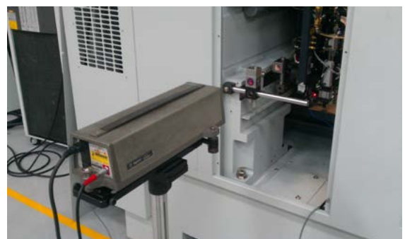
Figure 3 Measurement of Bilateral Amounts of Deformation of Saddle (1)
