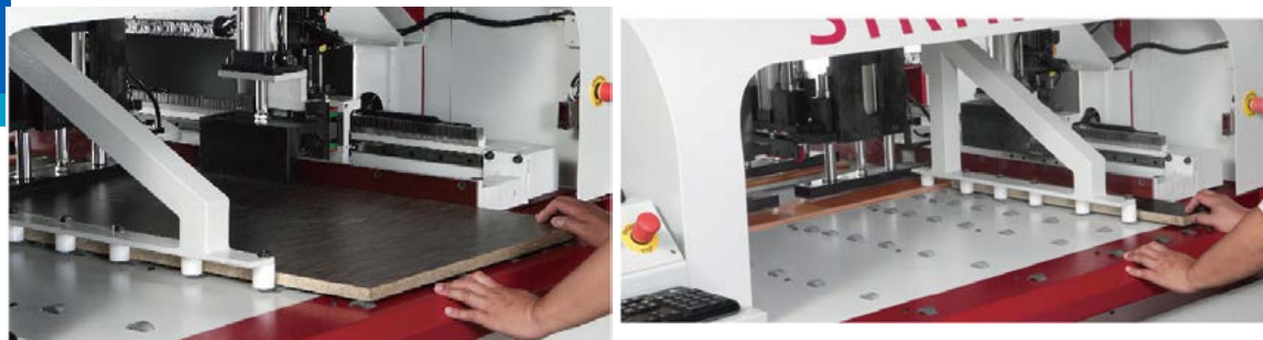
圖 4 板材定位零設定 Figure 4 None Setting Required for Positioning Plate Material
