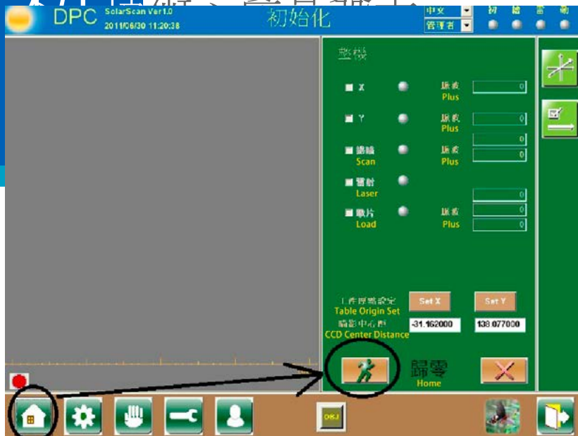
圖五 機台歸零 Figure 5: Setting the machine back to origin
