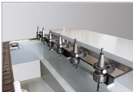
Automatic Tool Pick-up Station For rapid tool changing, saving time throughout the machining cycle.
