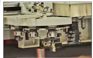
The automatic tool change system provides tool carousel or RanRob systems
